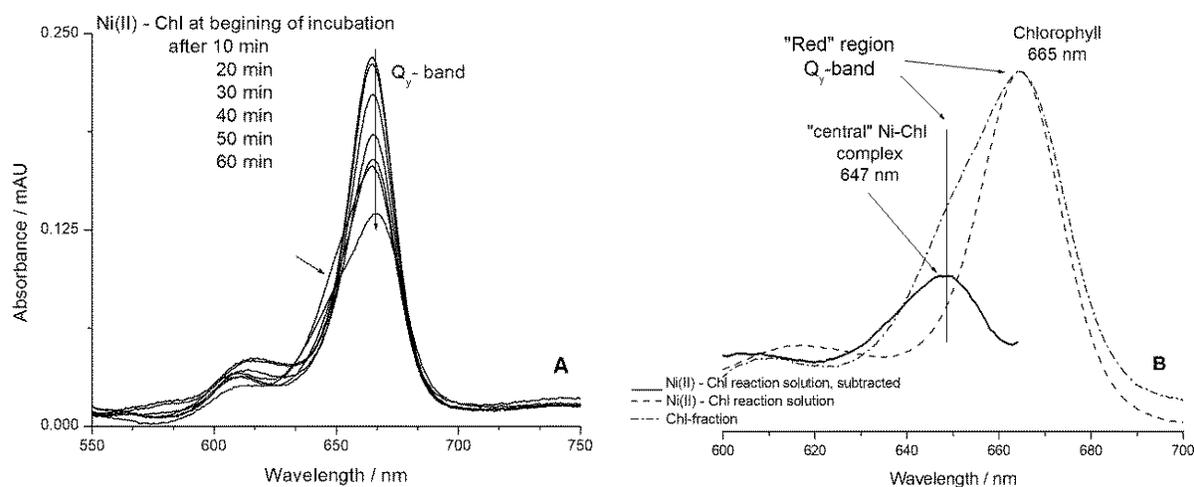
**Figure 2.** Absorption spectra of Ni(II)–chlorophyll reaction solutions in the “red” spectral region, following increasing periods of incubation, in 95 % ethanol (A). Absorption spectra of Chl in the “control” sample, Ni(II) – chlorophyll reaction solution (normalized to  $Q_y$  band absorption maximum) and assumed Ni-Chl complex, after 60 min of incubation (B).
