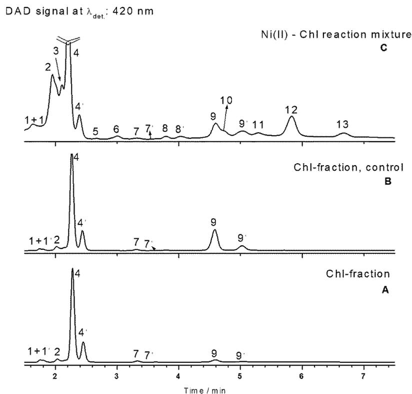
**Figure 3.** The UHPLC-DAD chromatograms for the Chl-fraction (A), “control” Chl-fraction (B), and Ni(II) – chlorophyll reaction solution (C), in 95 % ethanol after 60 min at 40 °C, recorded at 420 nm.
