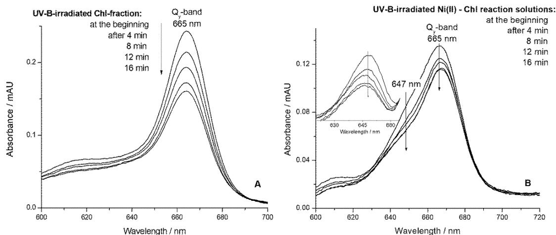
**Figure 4.** Continual UV-B irradiation induced degradation of chlorophyll fraction and Ni(II) – chlorophyll reaction solutions in 95% ethanol – changes in the absorption spectra during time exposure to UV-B irradiation (**A** and **B**, respectively); the corresponding spectra of assumed Ni-Chl complexes obtained by subtraction method, were shown as the increment of Figure 4B.
