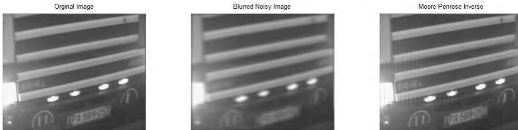
Figure 5.3.11. Removal of blur, caused by "salt and paper" noise and Gaussian function ( $l_c = 25$ ,  $l_r = 40$ ).
