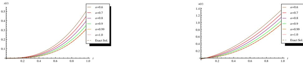
Figure 7: The approximated state  $x_5(t)$  and control variable  $u_5(t)$ , as a function of time  $t$  (Example 6.4).
