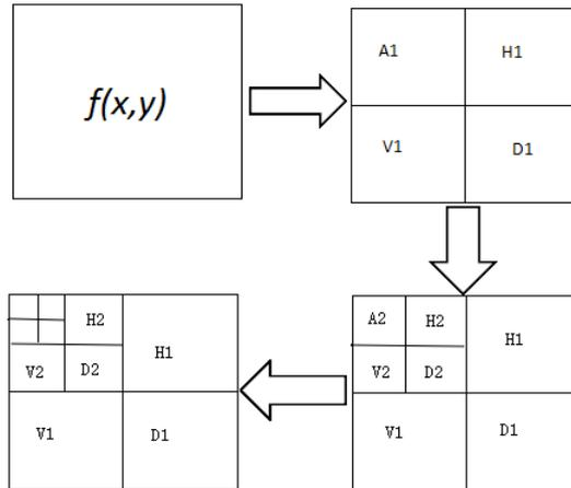
Figure 1: The Tower Structure of Image Wavelet Decomposition.
