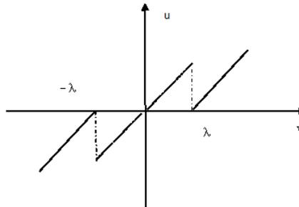
Figure 3: soft threshold function
