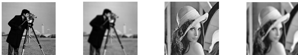
Figure 1: Original images: cameraman(left), lena(right), and their observed images with PSNR 21.3673 dB and 23.8492 dB, respectively.
