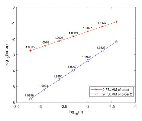
Figure 5: Errors and order of convergence for Example 2 at t = 1 for v = 1.6 and  $h = \frac{1}{25}, \frac{1}{50}, ..., \frac{1}{1600}$ .
