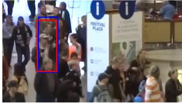
Figure 5: A detected bounding box D_i (in red) with an original confidence score of 0.35. A predicted bounding box (in blue) after not matching the tracklet T_j for 27 frames. For the given tracklet, threshold \beta_j = 0.8 . Since \text{IoU}(D_i, T_j) = 0.83 \geq \beta_j , the c_{d_i} is increased, and D_i will not be discarded.
