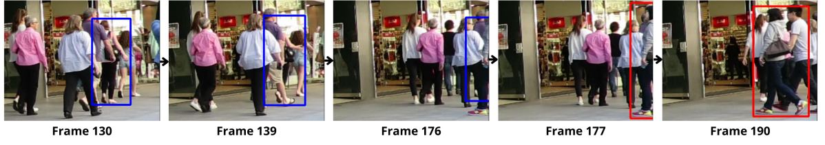
Figure 4.5: Example of an identity switch after occlusion between frames 139 and 176. The person moving to the right is incorrectly replaced by a person moving to the left. The gap should therefore not be interpolated, and the trajectory should be split.
