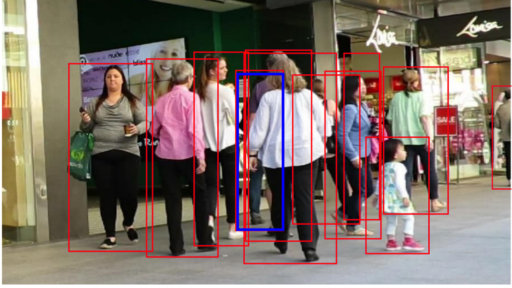
Figure 3.2: Detecting likely objects based on IoU value. Predicted tracklet bounding boxes are shown in red. The blue bounding box is the detection with the low confidence score, which is increased based on high IoU with the predicted bounding box.
