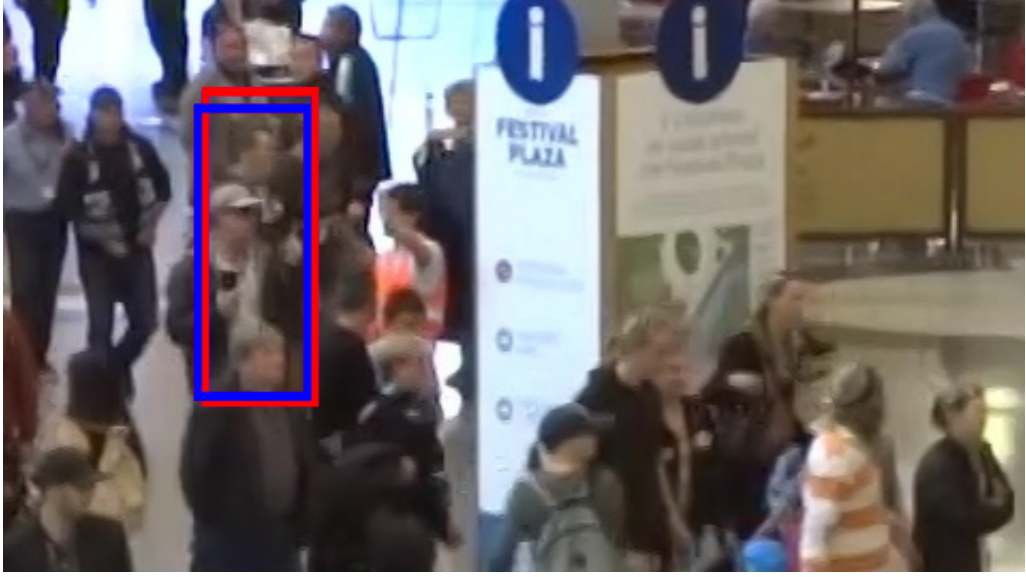
Figure 4.4: Example of varying similarity threshold. The detected bounding box D_i , shown in blue, has original confidence score 0.35. The predicted bounding box, shown in red, corresponds to a tracklet that has not been matched for 27 frames. The threshold for this tracklet is \beta_j = 0.8 . Since \text{IoU}(D_i, \hat{T}_j) = 0.83 \geq \beta_j , the confidence score c_{D_i} is increased, and D_i is retained for association.
